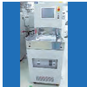
P-CVD1 samco PD-220NL Plasma CVD 1 samco PD-220NL
