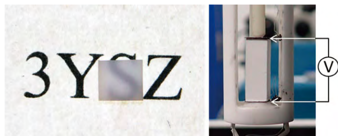
3mol%Y 2 O 3 -ZrO 2 ceramic by HAfS flashing technique at 1200°C for only 5min.
