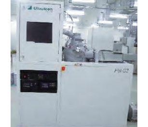
ALD(プラズマ式/サーマル式) Ultratech/CambridgeNanoTech Fiji G2 Atomic layer deposition system (Plasma/Thermal) Ultratech/CambridgeNanoTech Fiji G2
