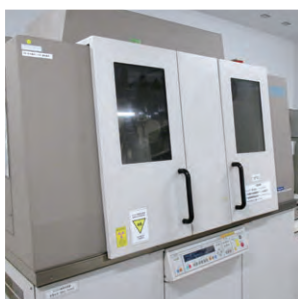
X線回折装置 RINT2500TTR X-ray diffractometer RINT2500TTR
