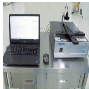
光干渉膜厚計(自動マッピング式) FILMETRICS F50 Automated Thickness Mapping Systems FILMETRICS F50
