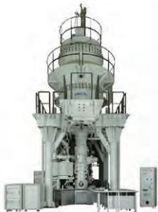
反科学超高压走査透過電子顕微鏡 JEM 1000K RS Reaction science high voltage scanning TEM JEM1000K RS
